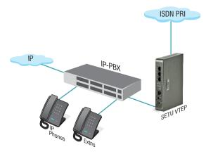
SETU VTEP connects an IP-PBX system to digital T1/E1 or PRI network. It enables the IP-PBX users to place calls over wide-spread ISDN PRI network. SETU VTEP can be connected directly through the LAN or remotely over the public IP network.
