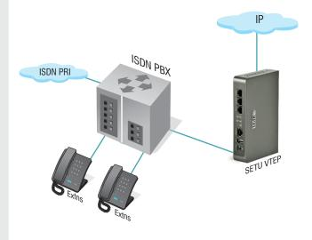
SETU VTEP transparently integrates with existing ISDN PBX using T1/E1 or PRI signaling to provide VoIP connectivity to existing PBX users. Programmable TE/NT modes ensure a hassle-free integration. Dedicated ports for network clock sync avoid synchronization errors and guarantee superior voice quality.
