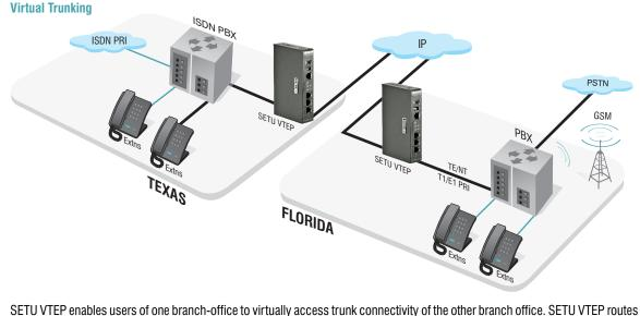
SETUVIEP enables users of one branch-office to virtually access trunk connectivity of the other branch office. SETUVIEP routes the call over cost-effective IP network till the last mile of termination and facilitates users at one location to access the local ISDN connectivity of remote branch-office to further reduce inter-network call charges.
